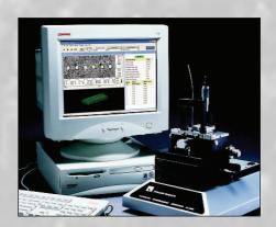
The AC-3005 provides repeatable angle measurements, certified to 0.01°, and radius of curvature measurements accurate to within 10% across the selected region of interest. Fiber height measurements and differential fiber height have been shown to be repeatable to within 40 nanometers.
